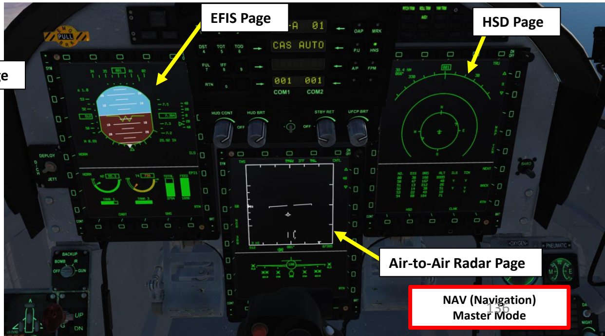
T1: MMS (Master Mode Switch) • UP: AA (Air-to-Air Intercept) • MIDDLE: NAV (Navigation) • DOWN: AG (Air-to-Ground)
