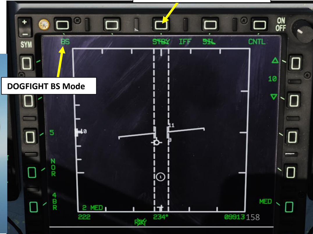
Radar Standby/ON Selector (STBY Crossed Out = Radar ON)
